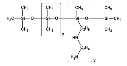
The amine-alkyl functionality of *GP-988-1 SILICONE FLUID* provides a versatile reaction site for the synthesis of a wide variety of silicone/organic copolymers, which may be tailored for use in textiles, coatings, car polishes and many other applications. The presence of polar amine groups also gives greater affinity to many substrates, suggesting uses of *GP-988-1* in lubricant, coating and mold release formulations.
