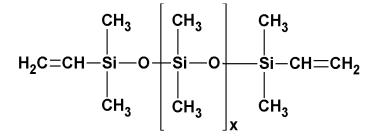
The vinyl functionality of *GP-977 SILICONE FLUID* provides a reactive site for cross-linking by ultraviolet or heat accelerated free radical cross-linking reactions.
