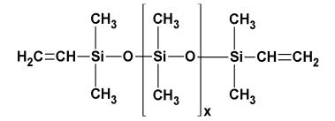
The vinyl functionality of *GP-908 SILICONE FLUID* provides a reactive site for cross-linking by ultraviolet or heat accelerated free radical cross-linking reactions.
