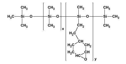
*GP-712* Can be cured with standard epoxy curing agents, or with cationic UV photo initiators in radiation cure applications. Cured surface coatings are used as release backings for pressure sensitive labels.
