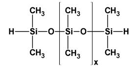
The silicon - hydrogen groups of *GP-536* provide a reactive site, allowing reaction with a variety of materials containing vinyl groups or with hydroxyl functional polysiloxanes in combination with heat or metal catalysts.
