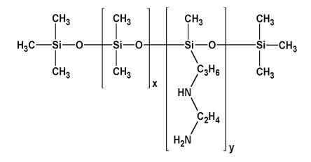
The amine-alkyl functionality of *GP-342 SILICONE FLUID* provides a versatile reaction site for the synthesis of a wide variety of silicone/organic copolymers, which may be tailored for use in textiles, coatings, car polishes and many other applications. The presence of polar amine groups also gives greater affinity to many substrates, suggesting uses of *GP-342* in lubricant, coating and mold release formulations.
